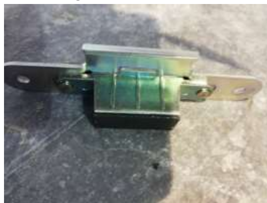
10) Top keep (identical to bottom keep) showing intumescent
