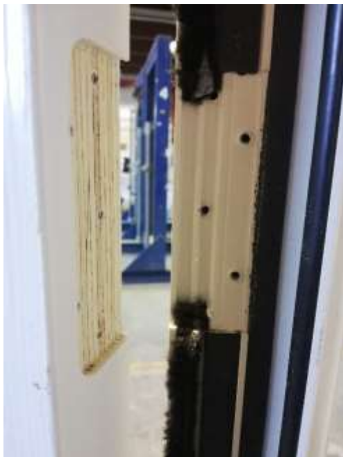
5) Hinge blade seal interruption
